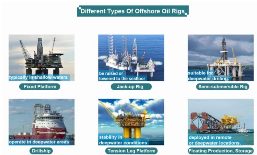
Fig.II.6: Classification des appareils de forage
