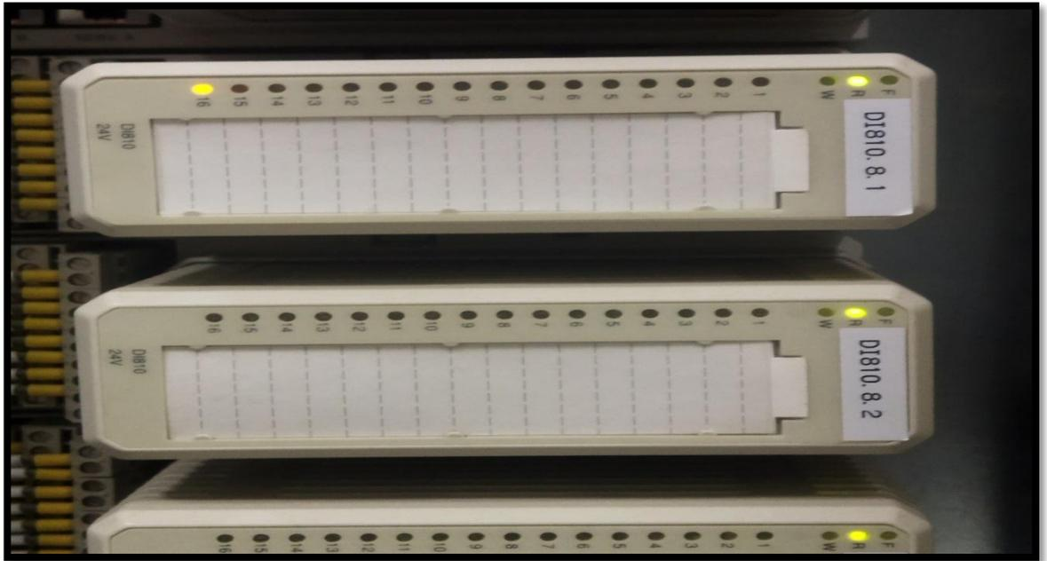
Figure III.17: module DI810 S800.[2]
