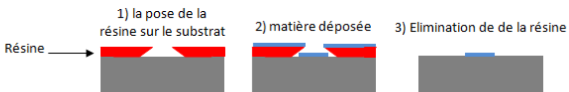
Figure II. 30 : Principe de la technique Lift-off.
