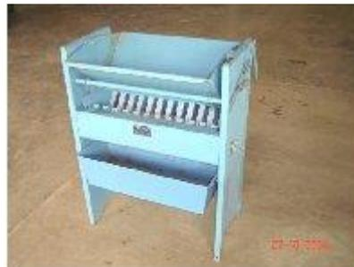
Figure. 22 Echantillonneur
