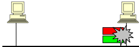
3- Station 2 sends a frame t at time \tau : a burst signal is created.
