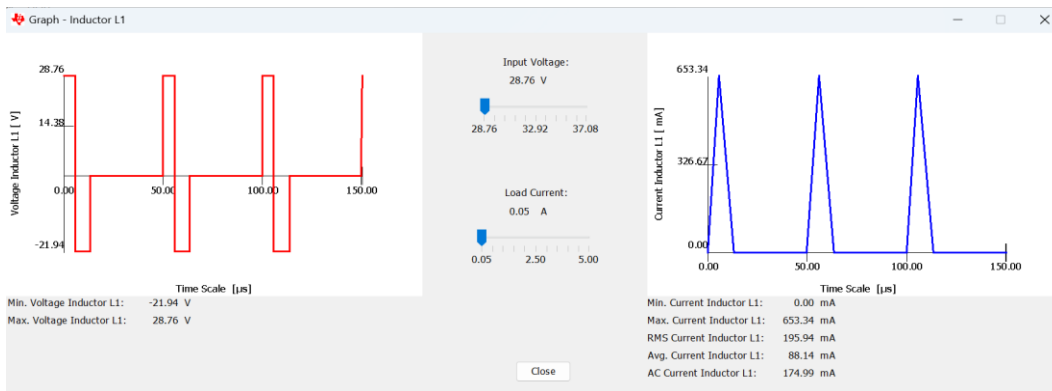
Figure II.18: Topology Window for Boost ‘Inductor current ripple: \Delta_iL=30\% ’
