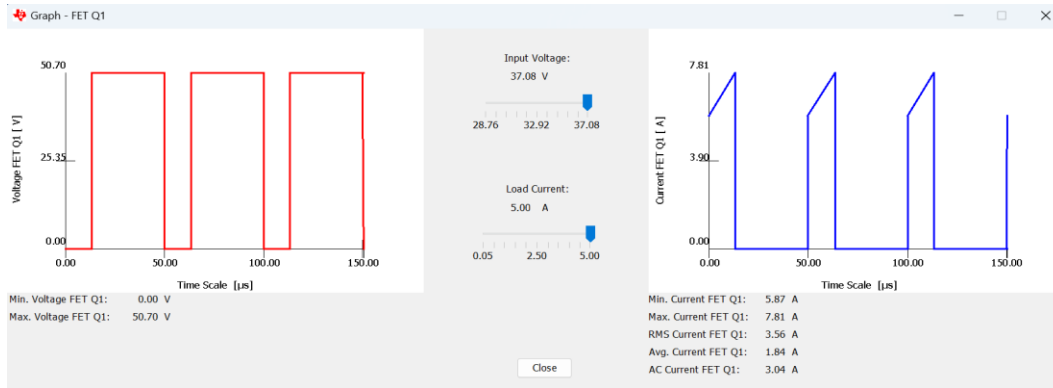
Figure II.19: Sizing results waveforms of the current and voltages: (a) for Inductor Input voltage=28.76 V / Load current = 0.05 (A), (b) for Inductor Input voltage=37.08 V / Load current = 5 (A), (c) for Mosfet Input voltage=28.76 V / Load current = 0.05 (A), and: (d) for Mosfet Input voltage=37.08 V / Load current = 5 (A).
