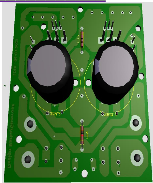
Figure II. 24:(a) PCB layout design diagram and (b) design 3D visualizer.
