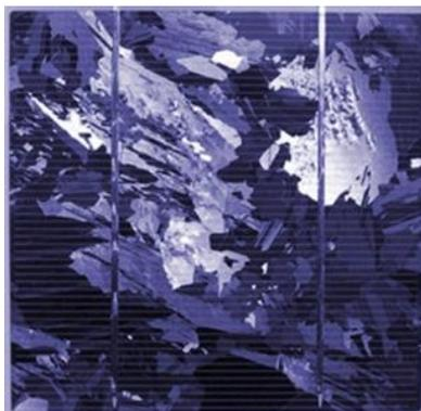
**Figure 1.4 :** Cellule photovoltaïque poly-cristalline.
