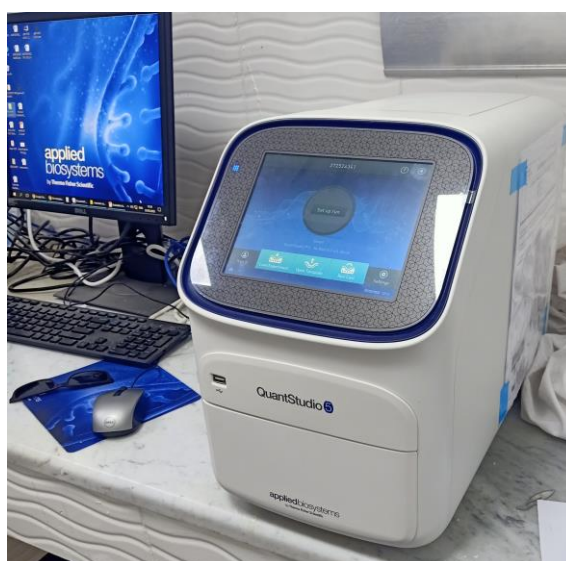
Figure 21: Thermocycleur QuantStudio™ 5 d'Applied Biosystems™.
