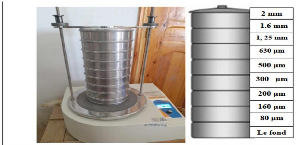
*Figure III. 1: machine de tamisage*
