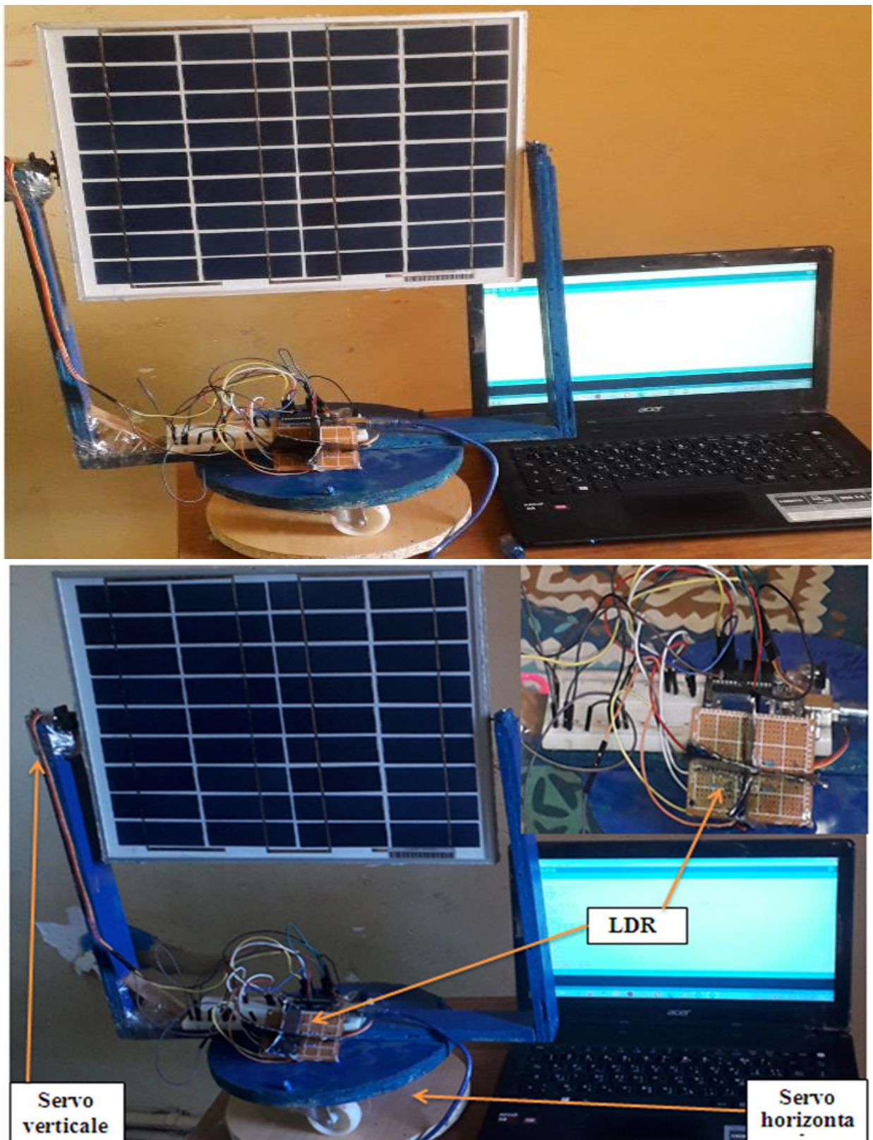
Figure III.41: Tracker solaire double axe.
