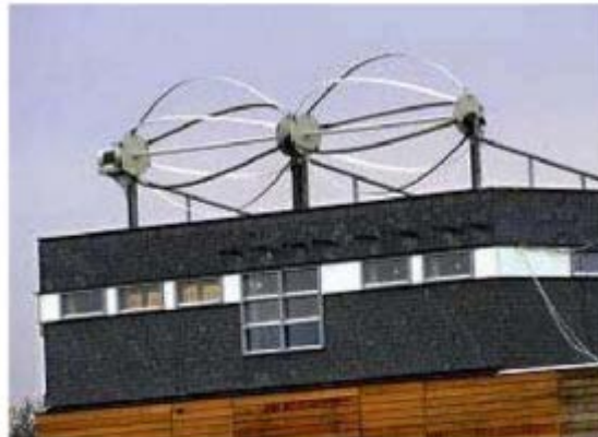
Fig. I.3: Eolienne de type Darrieus (Wind Wall) [5]
