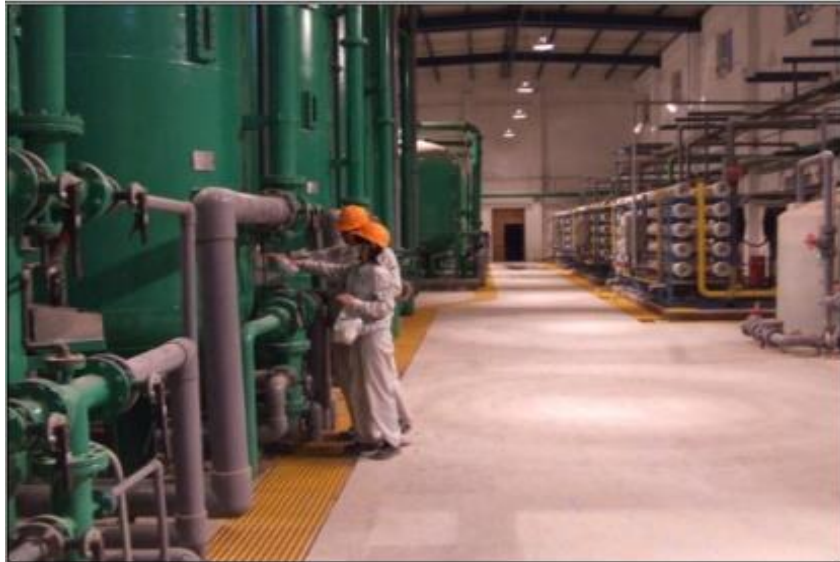
Figure I.18 Reverse osmosis filtration
