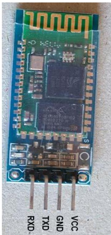
Figure III.40. Module Bluetooth HC-06.
