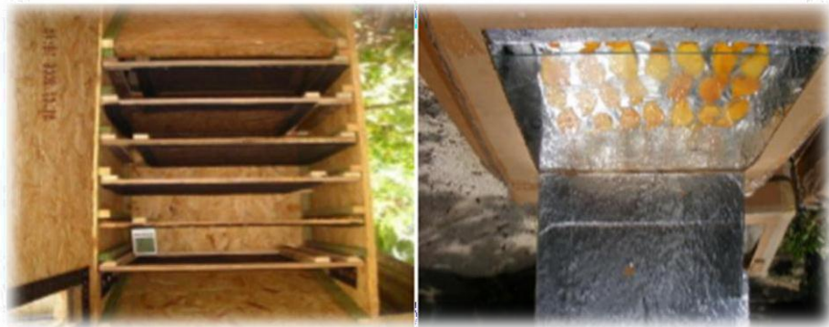
Figure III.21. Chambre du séchoir solaire indirect [33]
