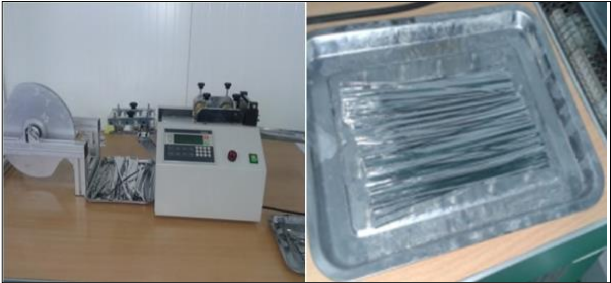
Figure II.14: Cutting the welding tapes
