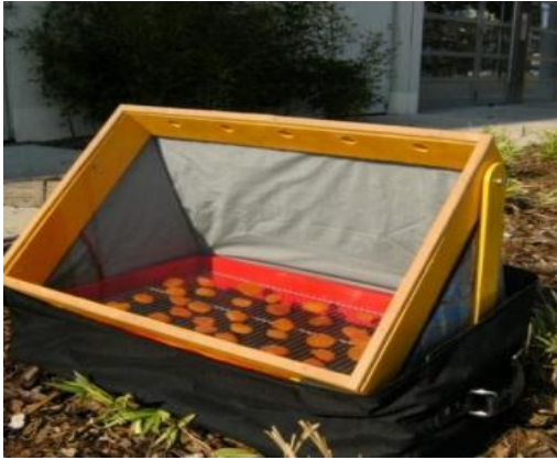
Figure II.3: Exemples des séchoirs solaires directs simples. [12] [11]
