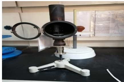
Figure III.10: Méthode ASTM D 1322.
