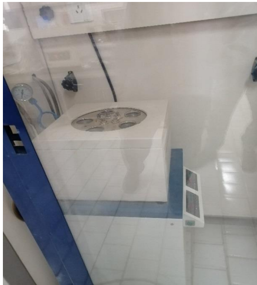
Figure III.15: Méthode ASTM D 381.
