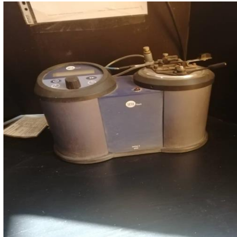
Figure III.9: Méthode ASTM D 3828.
