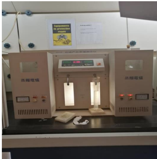
Figure III.7: Méthode ASTM D 86.
