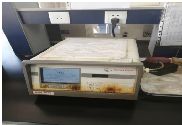
Figure III.8: Densimètre DMA 4500 NORM, ASTM D 4052.
