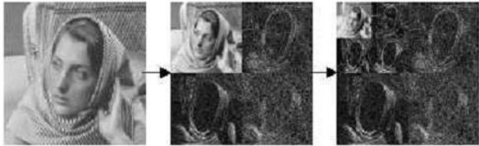
Figure 11: Example of Dyadic decomposition.
