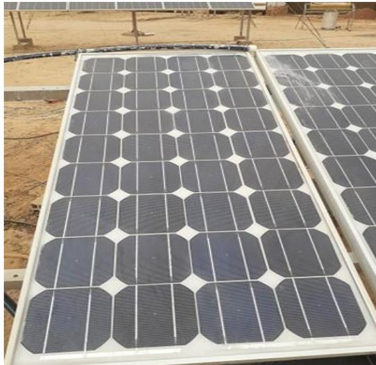
Figure IV.2: Modules testés ISOPHOTON I-75/12 (1, 2, 3)
