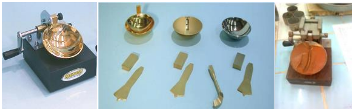
Figure II.11: Appareil de Casagrande (cas a, b) [9].
