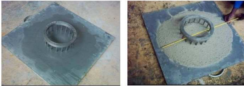
Figure I.11 : Essai J. Ring [13].
