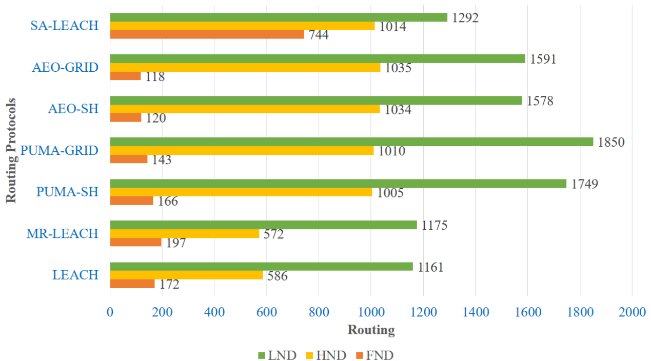
Figure 5.13: Comparison of FND, HND, and LND across different routing protocols with BS inside.
