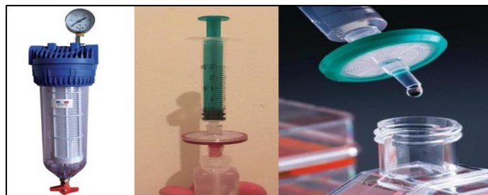
Figure 9: pressure filtration devices
