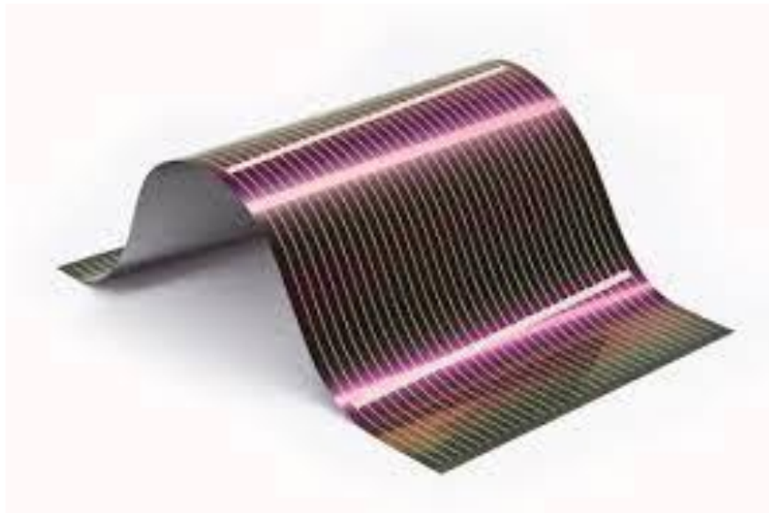
Figure 1.17: Thin-film solar cells that are based on copper indium gallium selenide
