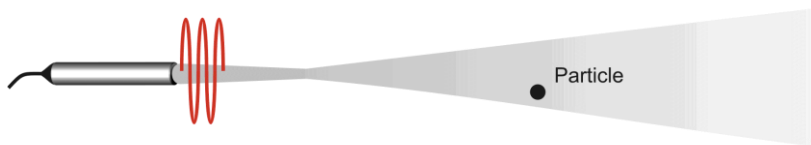
Figure 4.7: Pulsed ultrasound velocimetry principle
