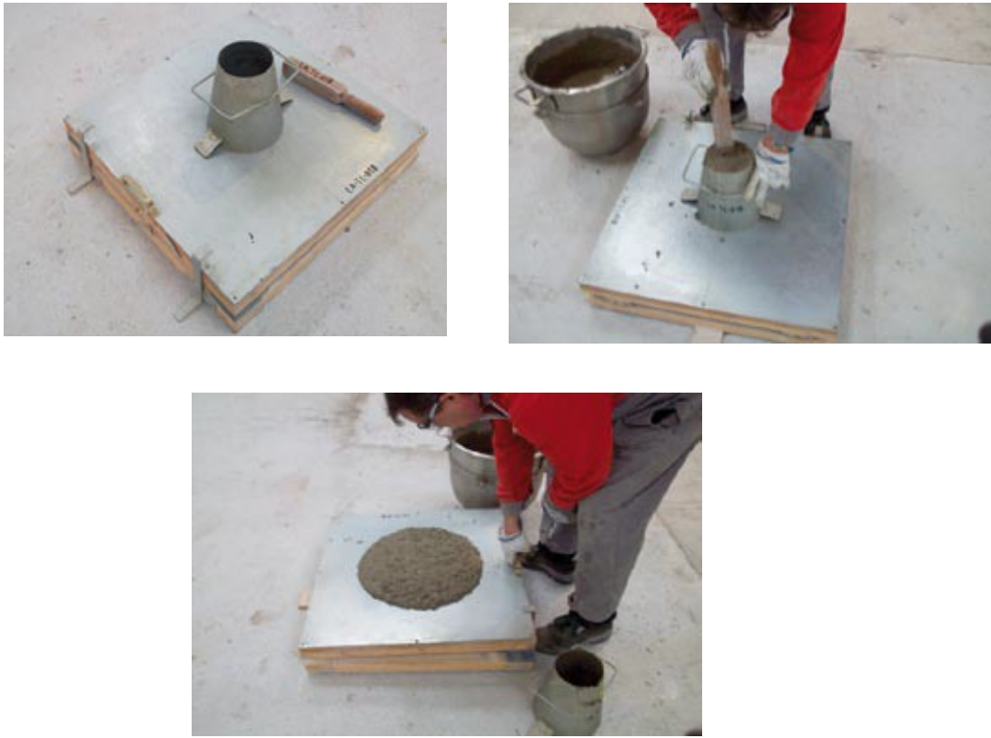
Figure III-2: Spread test using the Abrams cone
