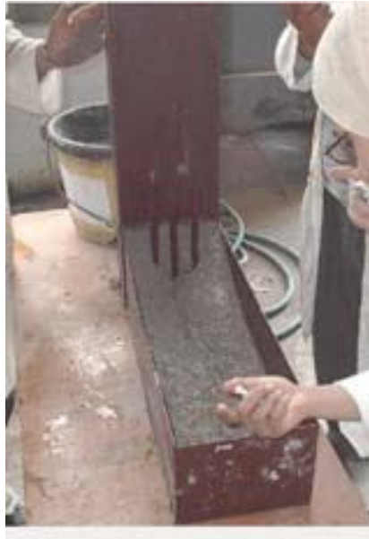
Figure III-5: Realisation of L-box test
