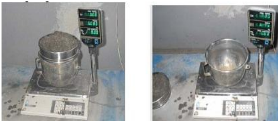
Figure III-3: Sieve Stability Test
